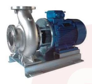
The installation dimension of the pump accord with ISO 2858: Design pressure up to 1.6MPa. Seal cavity construction is suitable for both of mechanical seal and soft packing seal; All the chemical pump parts are stainless steel precision casting. According to the requirement of liquid medium, we can supply the material configuration such as Cast Iron, Stainless steel and copper alloy and etc.
