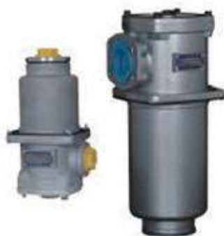
RF Tank Mounted Return Filter Series Flow rate: 60-1300L/min Pressure: 1MPa Precision: 1-30 \mu m Dia.: 20-100mm Connecting: Thread, Flange Element Model: LH Series
