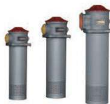
RFA Tank Mounted Mini-type Return Filter Series Flow rate: 25-1000L/min Pressure: 1.6MPa Precision: 1-30 \mu m Dia.: 15-90mm Connecting: Thread, Flange Element Model: FAX Series
