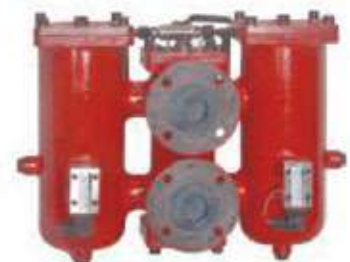
SRLF Duplex Return Line Filter Series Flow rate: 60-1300L/min Pressure: 1.6 MPa Precision: 1-30µm Dia.: 25-100mm Connecting: Flange Element Model: SFX Series
