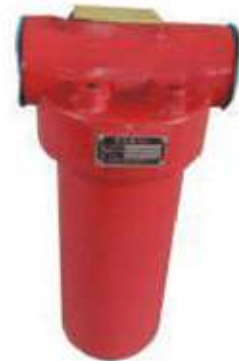
GU-H Tank Mounted Pressure Line Filter Series Flow rate: 10-630L/min Pressure: 32 MPa Precision: 3-40µm Dia.: 15-55mm Connecting: Thread, Flange Element Model: GX Series
