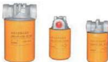
Spin Line Filter Flow rate: suction: 25-80L/min return: 60-320L/min Maximum Pressure: 0.7MPa Precision: 1-30 \mu m Connecting: Thread Element Model: SP (A, B) X Series
